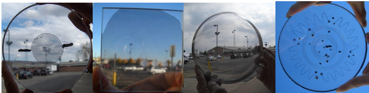
Figure 2 Examples of ALON window with internal RF Dipole Antenna (left); window and dome with embedded mesh (center) and ALON window with internal cooling channels (right)
